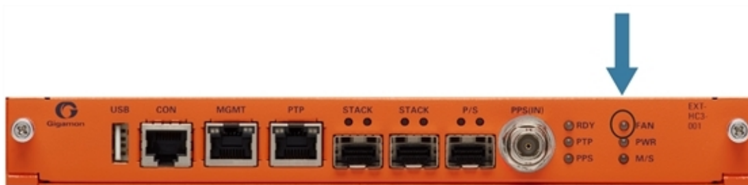
Figure 5 Global Fan LED Location on GigaVUE-HC3 Front
