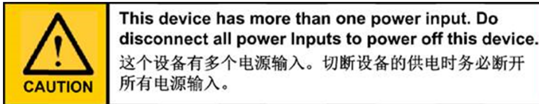
Figure 3 Power Caution Label
